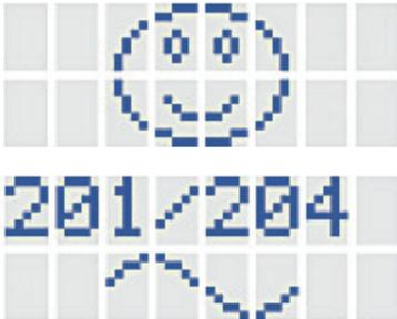
After 30 minutes, the “treatment complete” icon will appear as a smile face on the display—the device will beep twice and automatically shut off.
