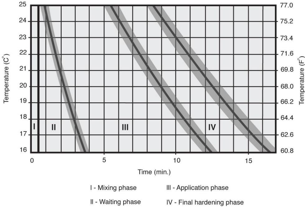
Handling and Setting Times vs. Temperature
