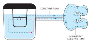
ICEMAN with dual pump recirculation technology. The DonJoy® IceMan® features a recirculation system that allows water warmed after flowing through the cold pad to be preserved and remixed with cooler ice water at a constant flow rate, providing consistent cool water distribution throughout the cold pad.
